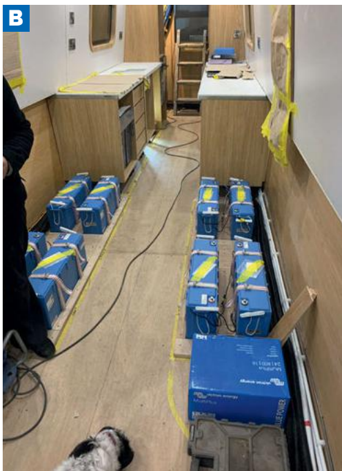
A A cover in the engine bay protects the electric motor frame and shorepower cable, as yet unused and still coiled. B The 200Ah 24V batteries being sized up before being fitted underneath the dinettes. C The electric cupboard has a mass of well-ordered cabling and components in a ventilated space. D At cruising speed the motor is running around 800rpm, drawing 40A (around 2kW). E The 6.5kVA low-speed diesel generator is quiet and can quickly recharge the battery bank, if required, as well as heat the hot water.
