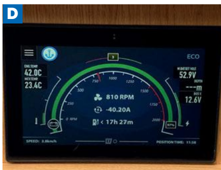
A A cover in the engine bay protects the electric motor frame and shorepower cable, as yet unused and still coiled. B The 200Ah 24V batteries being sized up before being fitted underneath the dinettes. C The electric cupboard has a mass of well-ordered cabling and components in a ventilated space. D At cruising speed the motor is running around 800rpm, drawing 40A (around 2kW). E The 6.5kVA low-speed diesel generator is quiet and can quickly recharge the battery bank, if required, as well as heat the hot water.
